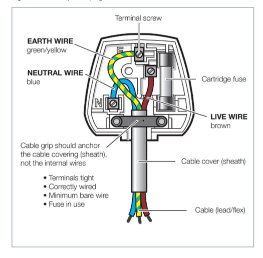
Figure 1 A correctly wired plug
